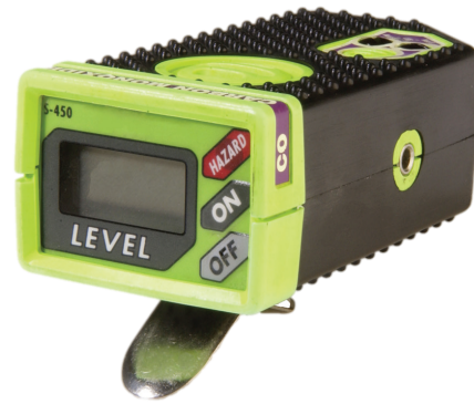
Figure 4-6: Portable CO gas detector. Source: Propane Education and Research Council.
